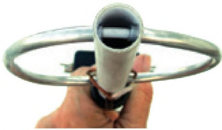
Figure 4 — Loop from the top end. Tune the loop by sliding the coax inner conductor and dielectric with your fingernail.
