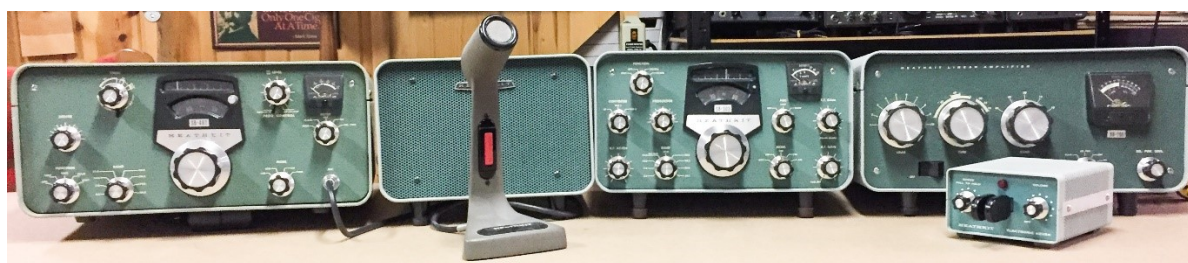
Heathkit SB-101 (successor to the SB-100) with SB-600 Speaker. Shown with HP-23 AC Power Supply mounted inside of the SB-600 (out of view) (W9MXQ Shack Photo)
