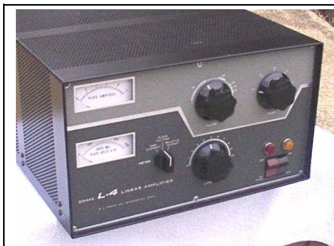
L-4 Linear Amplifier (Predates the L-4B) (2x 3-400z Eimac Tubes)
