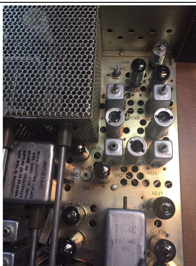
TR-4C – Cadmium Plated Chassis (In W9MXQ Drake Collection)
